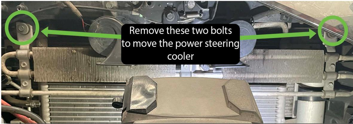
3.14. With the power steering cooler still connected to its flexible hoses, lower the power steering cooler down away from the upper radiator support. Be aware that the flexible section of the hoses aren't very long.
